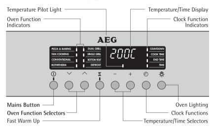
If the suggested temperature is not changed within approx. 5 seconds, the oven starts to warm up. The temperature pilot light indicates that the oven is warming up. When the temperature set is reached the temperature pilot light extinguishes. It will then cycle on and off to show that the temperature is being maintained
